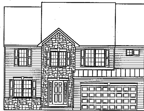
ELEVATION A-20 OPT. METAL ROOF SHOWN
