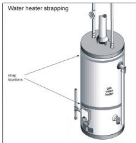
Illustration 9AE (Please note this diagram refers to two strap installations)
